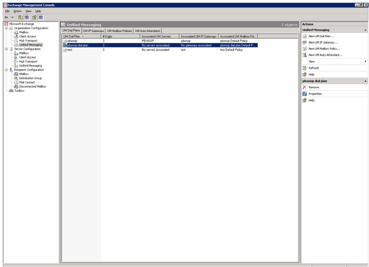
2. **Create a new unified messaging dial plan:** Using the Exchange management console, select Organization Configuration/Unified Messaging. Under actions select new UM dial plan. Name the dial plan 'pbxnsip' and set the 'number of digits in extension numbers' to 3. Click 'new' and
