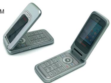
Pirelli's DP-M30 is a stylish Multimedia • Dual Mode Phone (Wi-Fi/GSM) Phone combining Tri-band GSM and VoWLAN telephony based on the SIP standard in a single device.
