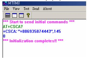
If the message "\*\*\* Initialization completes!! \*\*\*" shows up, then the communication between MT350 and the PC is OK, otherwise, you will see the message: "\*\*\* Timeout!! No response \*\*\*". In that circumstance, the serial port might not be assigned correctly, or it is occupied by other application program.
