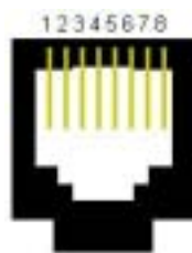
Figure 2-2 10/100 BASE-T Ethernet Port Pin Order
