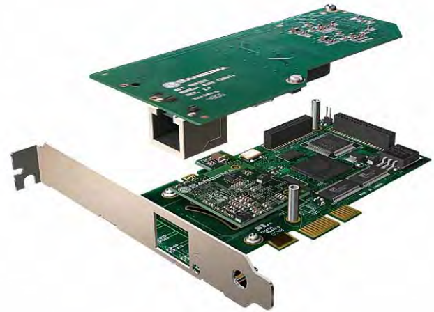
A101DE 1-port T1/E1/J1 shown with available echo canceller and PCI-Express interface
