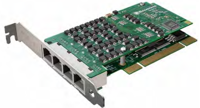
A108 8-port T1/E1/J1 shown with PCI Interface
