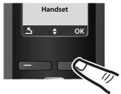
Press the bottom of the control key until the Handset menu item appears on the display.
