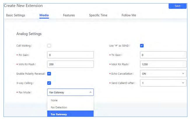
Figure 179: Configure Extension for Fax Machine: Analog Settings
