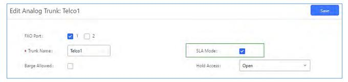
Figure 102: Enable SLA Mode for Analog Trunk
