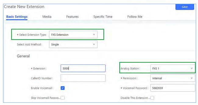
Figure 178: Configure Extension for Fax Machine: FXS Extension
