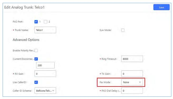
Figure 177: Configure Analog Trunk without Fax Detection
