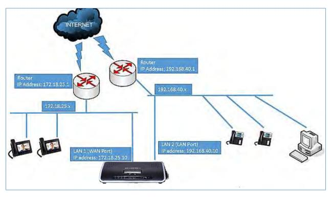
Figure 13: UCM6202 Network Interface Method: Dual
