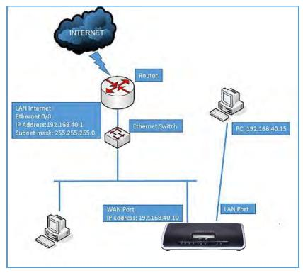
Figure 12: UCM6202 Network Interface Method: Switch
