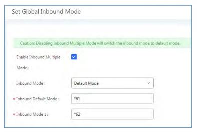
Figure 118: Inbound Route - Multiple Mode Feature Codes
