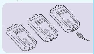
3. When the battery indicator bar stops scrolling, charging is complete. The text "Fully Charged!" is also displayed on the LCD screen, if the phone is off.
