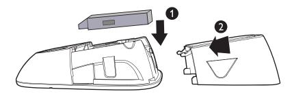
**Step 1:** Place the battery (with the label **THIS SIDE UP** facing up) into the battery compartment.
