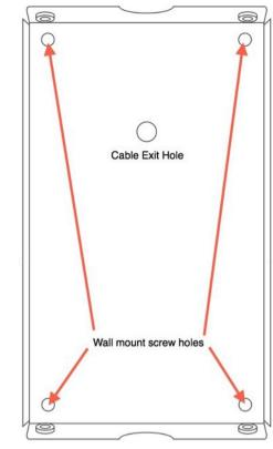
The wall mounting plate can be separated from the phone by unscrewing the four pin hex security screws at the rear of the case. A 15mm cable exit hole is provided to allow you to feed the ethernet cable from the rear of your phone.
