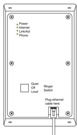
If power is available on the ethernet connection the green power LED will be illuminated followed by the Internet LED and the Link/Activity LED if there is access to the Internet on the network and there is a DHCP server. The Phone LED will remain off until you configure your SIP settings.
