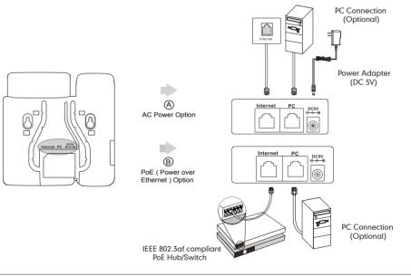
**Note:** If inline power (PoE) is provided, you don't need to connect the power adapter. Make sure the Etherne cable and hub/switch are PoE compliant.
