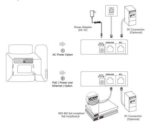
**Note:** If inline power (PoE) is provided, you don't need to connect the power adapter. Make sure the Etherne cable and hub/switch are PoE compliant.
