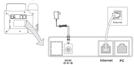
Note: If inline power (PoE) is provided, do not install AC adapter. Make sure the Ethernet cable and switch/hub are PoE compliant.
