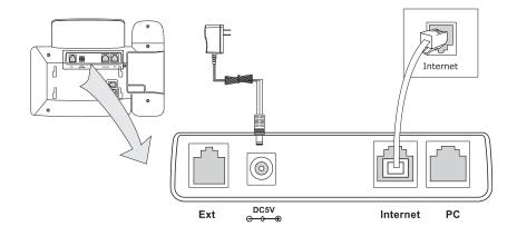
Note: If inline Power (PoE ) is provided, do not install the AC adapter. Make sure the Ethernet cable and switch/hub are PoE compliant.
