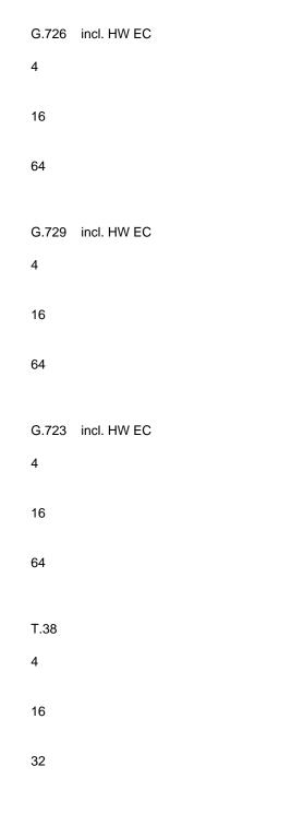
The card series consist of a baseboard and the so called LineInterfaces. Each baseboard can carry up to two LineInterfaces. The base boards are available as PCI or PCI express cards with the following channel densities:
